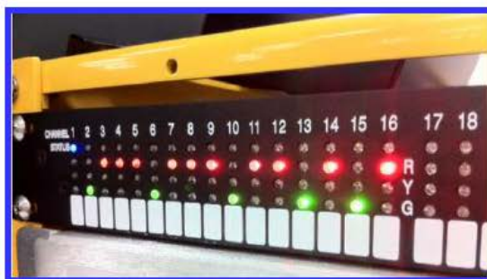
ADU 2220: CHANNEL STATUS blue indicator is on
