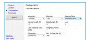
Figure 7-13: Configure Detector
