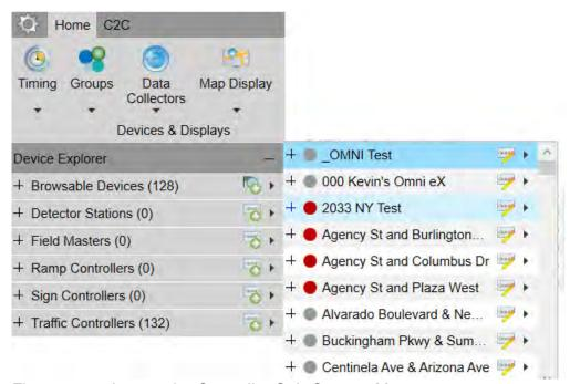
Figure 2-19: Access the Controller Sub-Context Menu
